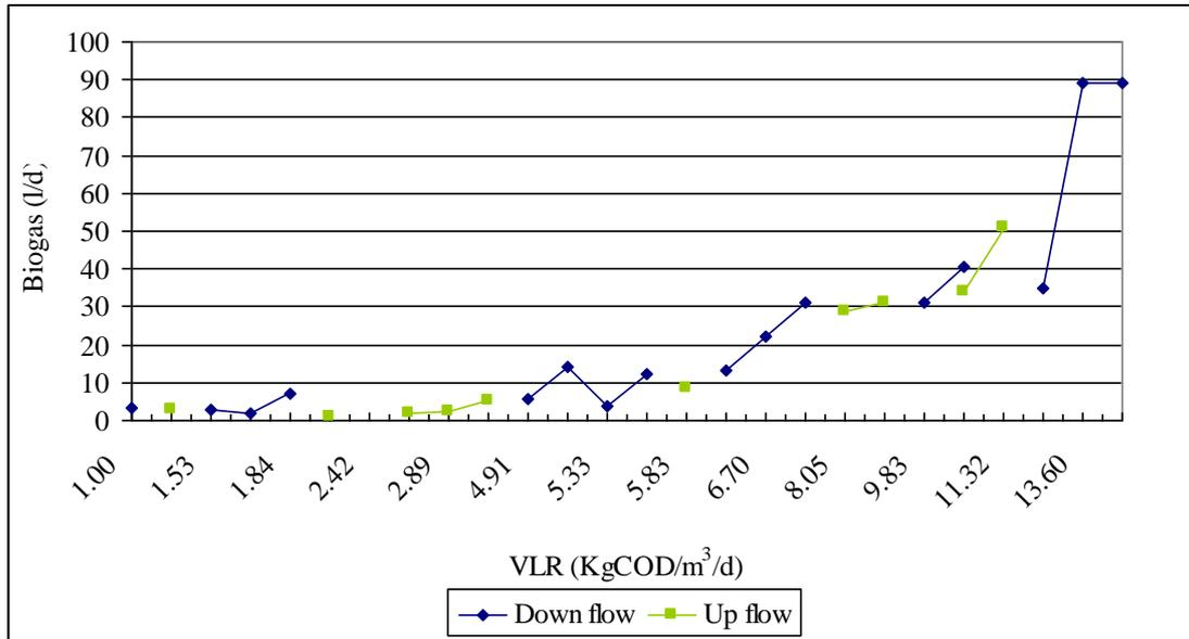
**Figure 2** Gas production in down flow and up flow configurations
