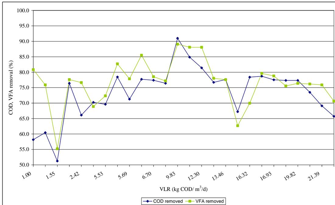
**Figure 4** COD&VFA removed as function of VLR in down flow configuration
