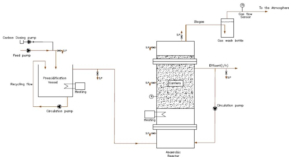
**Figure 1** Up flow Pilot Set up
