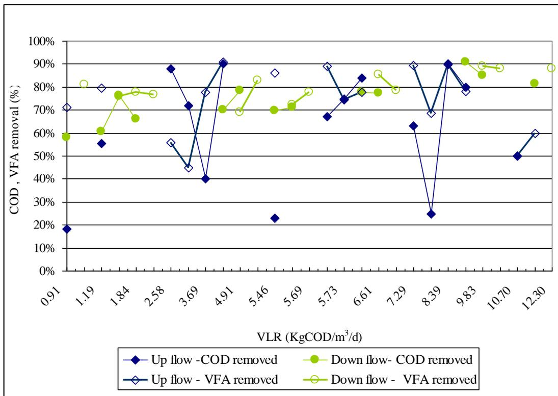
**Figure 3** COD&VFA removed as function of VLR in both configurations
