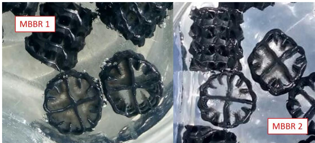
Figure 3: Carriers from MBBR 1 and 2 with biofilm
